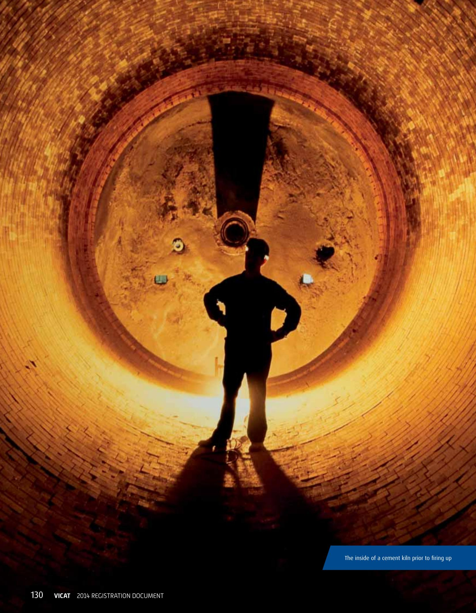
The inside of a cement kiln prior to firing up
