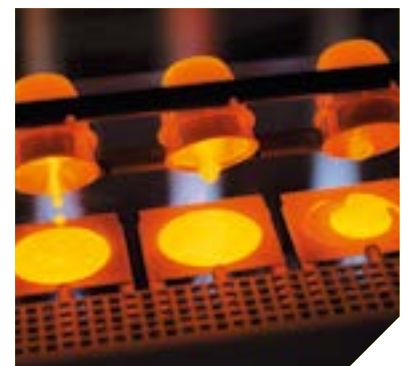
— Preparation of fused beads for X-ray fluorescence analysis by the materials and microstructures laboratory in L'Isle d'Abeau (France).
