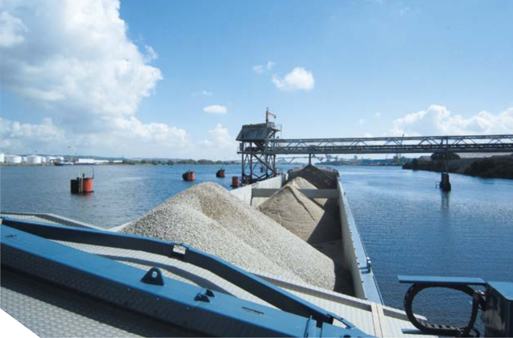
— River barges transport sand and gravel to the concrete batching plant in Gennevilliers (France).
