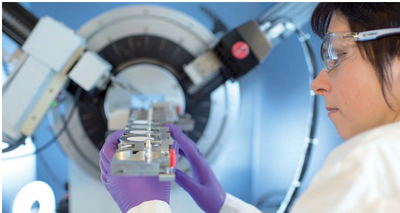
▲ Examination by means of X-ray diffraction using a high-speed detector in the materials and microstructures laboratory at the Louis Vicat technical center in L'Isle d'Abeau (France).
