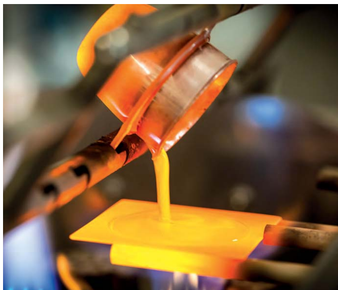
▲ Preparation of fused beads for X-ray fluorescence examination in the materials and microstructures laboratory at the Louis Vicat technical center in L'Isle d'Abeau (France).
