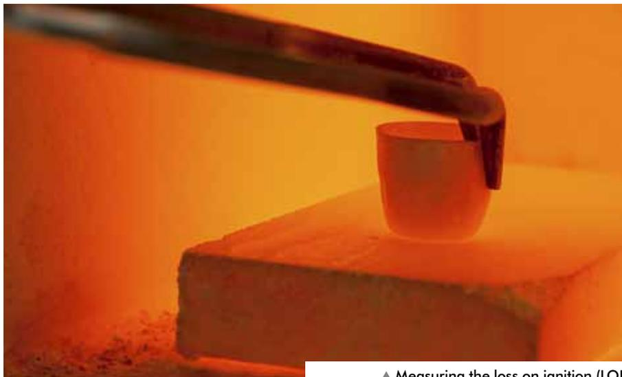
▲ Measuring the loss on ignition (LOI) of a cement to determine its limestone content.
