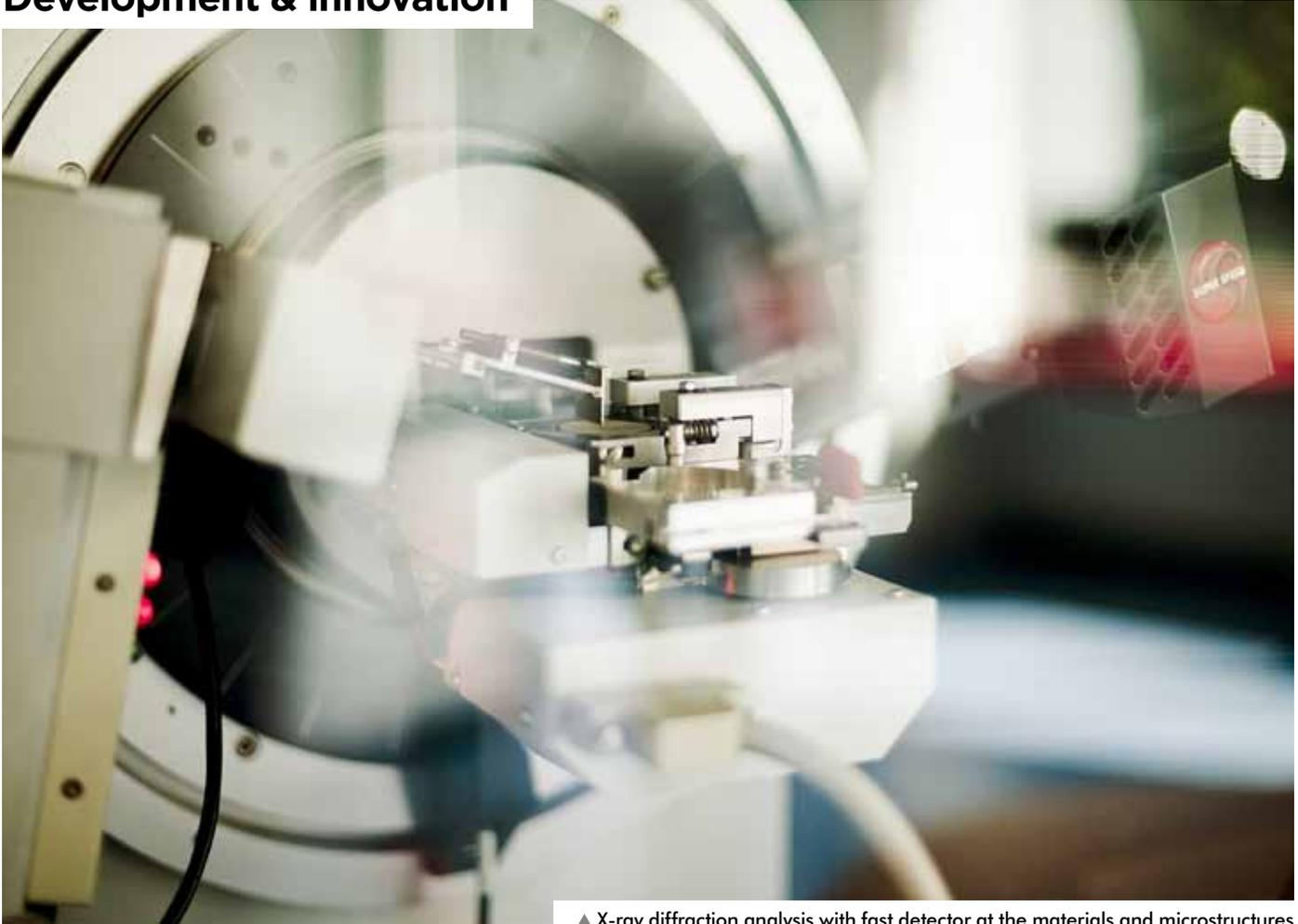
▲ X-ray diffraction analysis with fast detector at the materials and microstructures laboratory of the Louis Vicat technical center in L'Isle d'Abeau (France).
