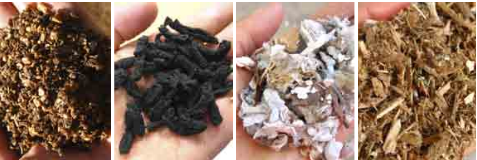
▼ Some of the different substitute fuels used to fire cement kilns: olive mill cake (OMC), dewatered sludge, shredded bulky waste (SBW), and wood chips.
